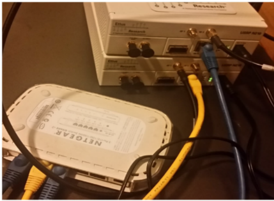
Figure 2. Connection of the USRPs to the Gigabit Ethernet Switch that is connecting the devices to the host.
