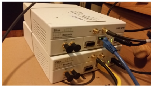
Figure 1. Two USRPs, each with one antenna connected to either RF1 or RF2.
