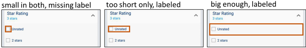
Fig. 16. A Checkbox element that, stand-alone, is too small in both dimensions and missing a label if without a contentDescription . If the clickable region includes the text label, then the element is too short only and labeled . Expanding the region to the full width and height of the row layout makes the element big enough . No modifications affect the visual appearance.
