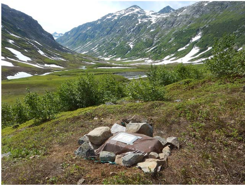
▲ Figure 4. Example of station setup at HLC2 just west of Redoubt Volcano and adjacent to the headwaters of Drift River. Large rocks pin the tarp onto the station box, which is the only visible component of the station. Photo taken after servicing the station on 20 July 2016; view is to the west. The color version of this figure is available only in the electronic edition.
