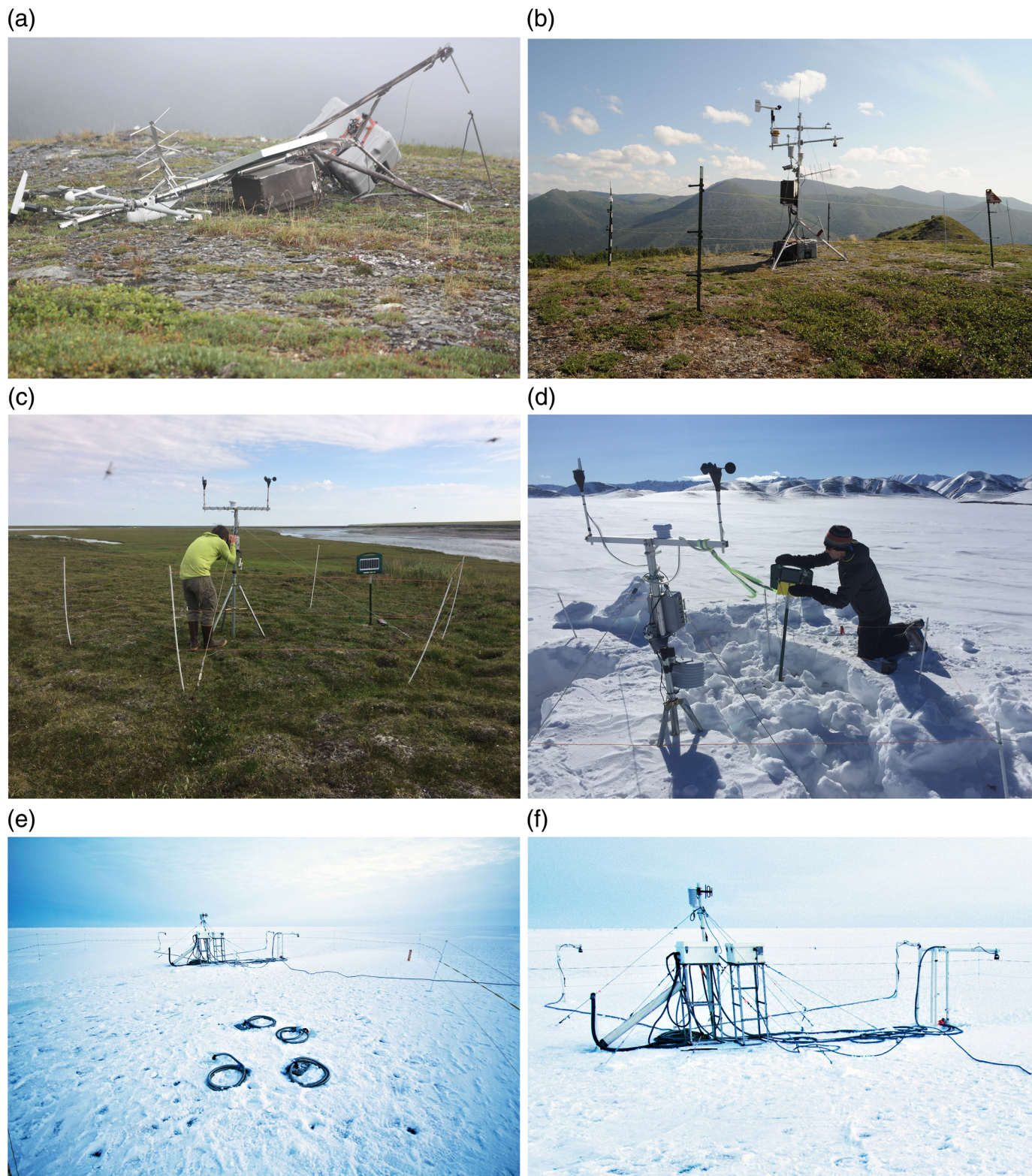
▲ Figure 10. Examples of electric fences installed to protect scientific measuring equipment in Alaska. (a) Bear damage to a National Park Service weather station at Salmon River in 2012. (b) Same site as in (a), but after electric fence were installed in 2013. No equipment has been damaged at this site since 2013. Photos provided by National Park Service (NPS). NPS weather stations are discussed in Sousanes, Hill, Bower, et al. (2017) , Sousanes, Hill, Johnson, and Miller (2017) . (c,d) U.S. Geological Survey (USGS) weather stations in northern Alaska. Photos provided by USGS, Alaska Science Center. (e) Sea ice monitoring station, offshore northern Alaska ( Druckenmiller et al. , 2009 ). Photo provided by Andy Mahoney. (f) Zoom-in on (e). The color version of this figure is available only in the electronic edition.
