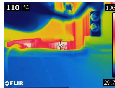
Fig. 6. Die temperature captured by thermal image camera during a 105^\circ\text{C} double pulse test
