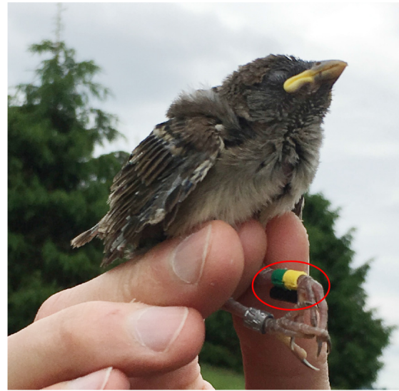
Fig. 16. RFID tagging arrangement of house sparrows studied in this work. A glass LF RFID tag is enclosed in heat-shrink tubing (the black cylinder) and attached to colored bands that encircle the leg of the house sparrow.
