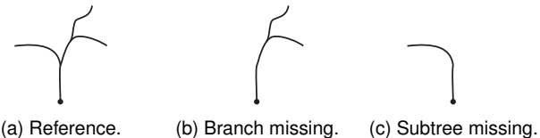
Fig. 9: Examples of incorrect traces (b,c) compared to a reference trace (a). Traces (b) and (c) score 0.875 and 0.5 with the DIADEM metric, respectively. The error in (c) misses a subtree containing more important features than are missed in (b), impacting subsequent analysis significantly, and is scored lower as a result.
