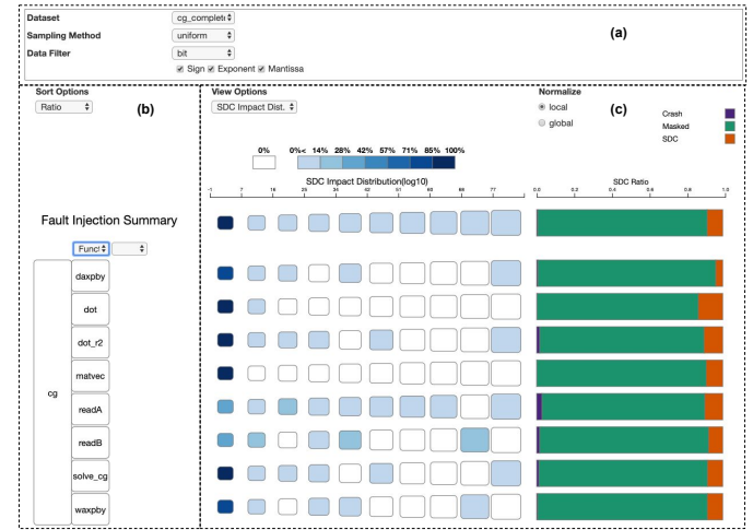
Fig. 3. Display of a CG benchmark dataset to compare the SDC impact and SDC ratio of across multilevel program components; (a) provides a set of filter and dataset options, (b) enables users to manually decide on a hierarchical structure of data that is presented in (c), and (c) is a composition of visual components to display SDC properties.
