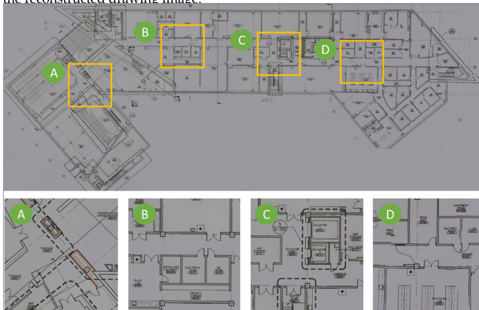
Figure 7. Drawing image reconstructed using DrawImgs. The four images on the bottom are magnified areas corresponding to the boxes on the drawing on the left.
