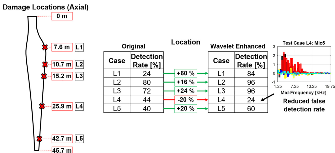
Fig. 14. Comparison of the overall damage detection performance obtained using a high pass filter and the adaptive WPD algorithm with respect to damage location.
