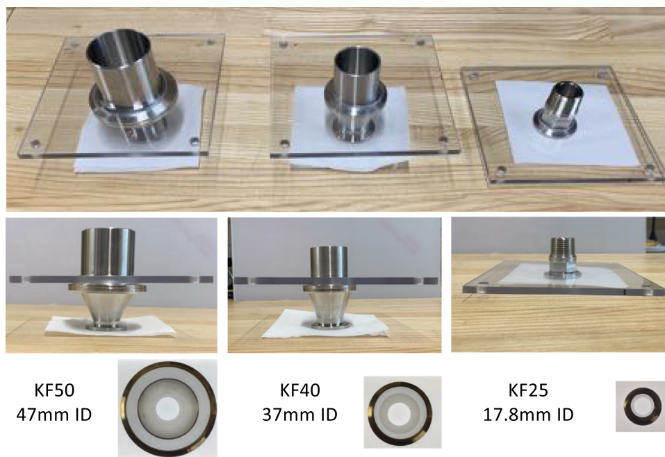
FIG. 8. Three sizes of KF flange permit adjustment of the face velocity for a given flow range.
