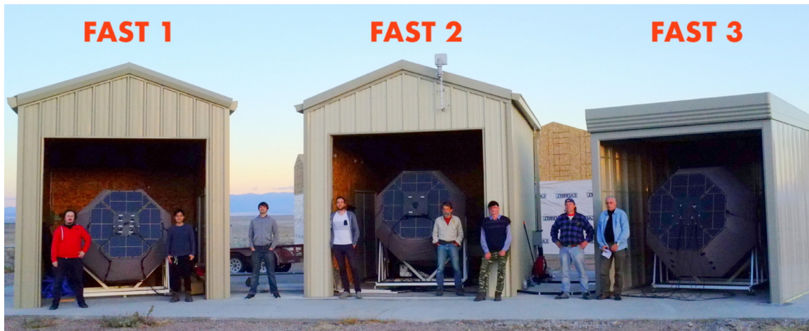
Fig. 6. The three FAST prototype telescopes installed at the Black Rock Mesa site of the Telescope Array experiment in central Utah, USA. The FAST All-Sky Camera (FASCam) and Sky Quality Monitor (SQM) can be seen attached to the roof of the central building (see Section 3.5 ).
