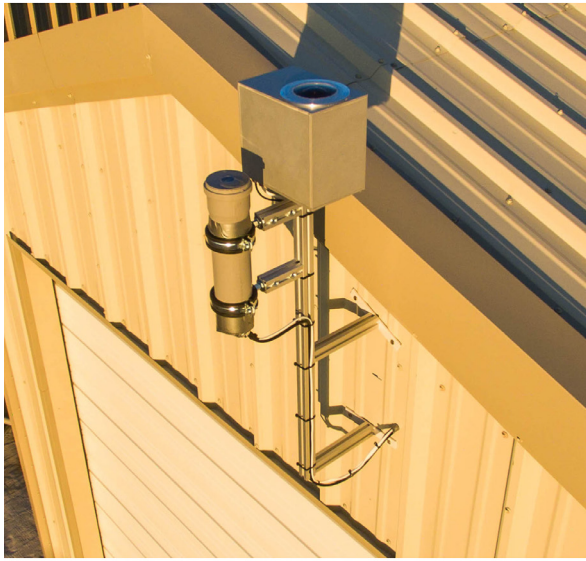
Fig. 12. Left: The FASCam and SQM installed on the central FAST telescope. Right: An example of a FASCam analysis. Identified stars are indicated with green circles, while stars that should be observable but are obscured by cloud are shown as red circles.
