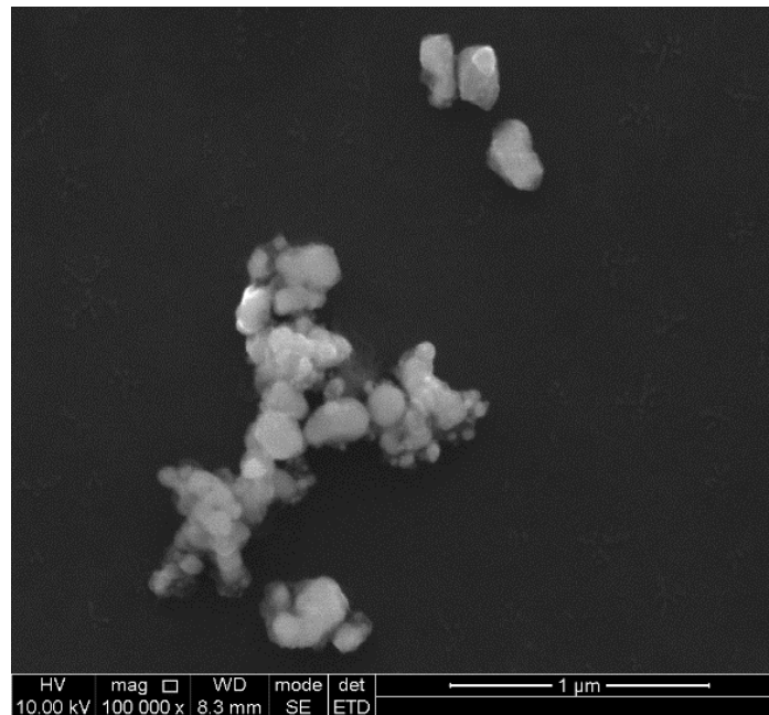
Fig.3. SEM microstructure of the Fe 50 Rh 50 sample.
