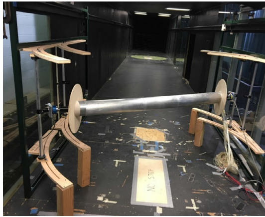
Fig. 4. Static test setup of yawed cable with end plates for pressure and force measurements.
