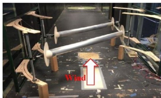
Fig. 3 Test setup of yawed smooth cylinders in tandem arrangement
