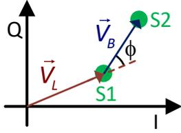
Fig. 7. Complex demodulated signals received by the reader.
