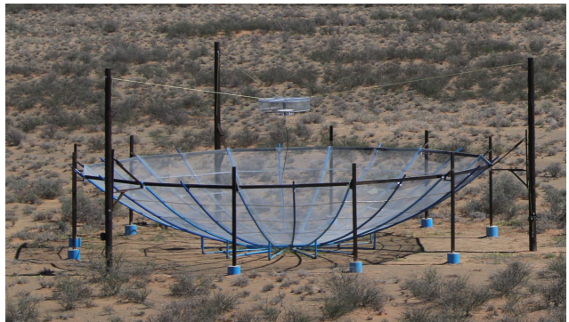
Figure 1. A single HERA antenna in the field with a cross-dipole feed surrounded by a cage hoisted to the antenna’s focal point. Image courtesy of Kathryn Rosie.
