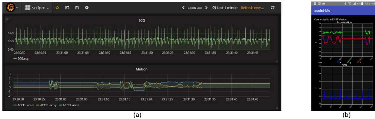
Fig. 4. Screenshot of the developed applications for data display: (a) Cloud interface displaying ECG and acceleration data; (b) Android application with ECG and acceleration data displayed.
