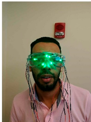
Figure 6. The FacePET wearable device. (a) Wiring sketch diagram for FacePET LEDs; (b) Schematic; (c) Goggles with LEDs and BLE microcontroller; (d) FacePET wearable prototype worn by a bystander.
