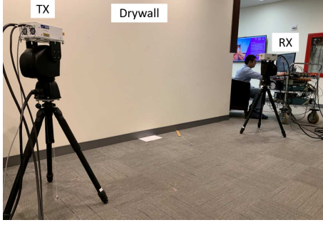
Fig. 1: Photograph of the reflection/scattering measurement setup. The reflected/scattered power of drywall was measured at a distance 1.5 m away from the wall, in angular increments of 10^\circ .
