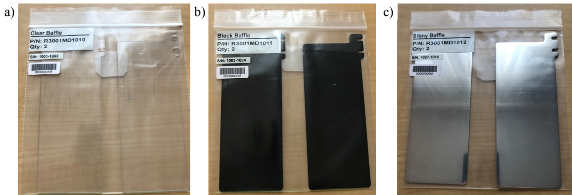
Figure 3. Three types of baffles. a) Transparent polycarbonate. b) Anodized black aluminum. c) Polished aluminum.
