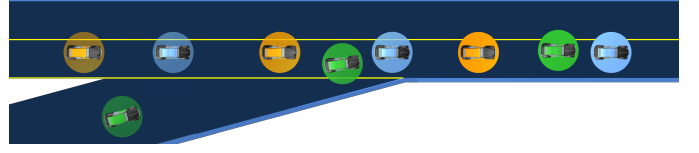
Fig. 3. On the left, the three cars at their nominal initial state. On the right, the three cars are standing at the desired final state. The green car has successfully merged in between the two other cars. The roadway boundaries are depicted in light blue.
