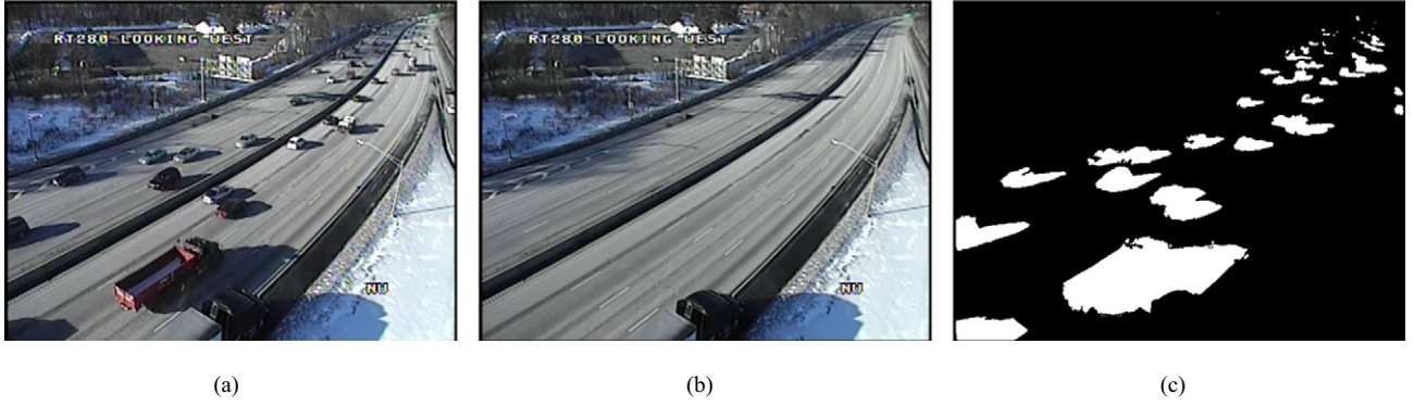
Fig. 1. (a) A video frame from an NJDOT traffic video. (b) The background derived using the GMM model. (c) The foreground (with shadow) detected using our new foreground detection method.
