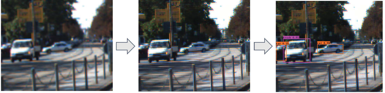
Figure 4: Detection of distant objects through ESRGAN. The left subfigure shows the region that is reported to contain objects. Enhancing the resolution of this region by ESRGAN, a higher-resolution image is obtained in the middle subfigure. Feeding the enhanced image into an object detection model, three vehicles are successfully detected in the right subfigure.
