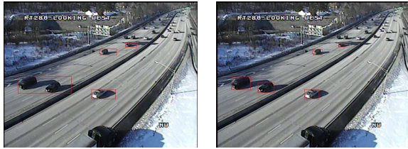
Fig. 6. The comparison of vehicle tracking performance between the tracking result without shadow detection(left) and the result with shadow detection(right).
