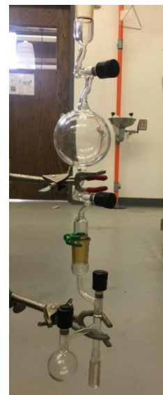
Figure S22: Cuvette with RB bulb attached, allowing for freeze-pump-thawing. A large, calibrated bulb is attached to the cuvette.
