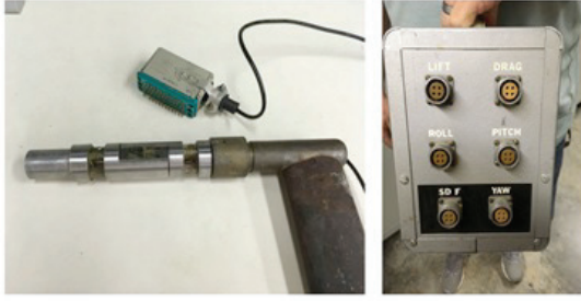
Fig. 4. 6DOF Sting Balance SB-100 model (left), strain gauge box converter (right)
