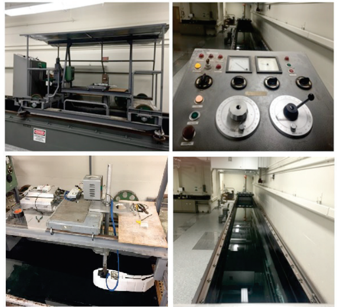
Fig. 3. Top: Towing carriage, control panel. Bottom: Installed MBE, towing tank
