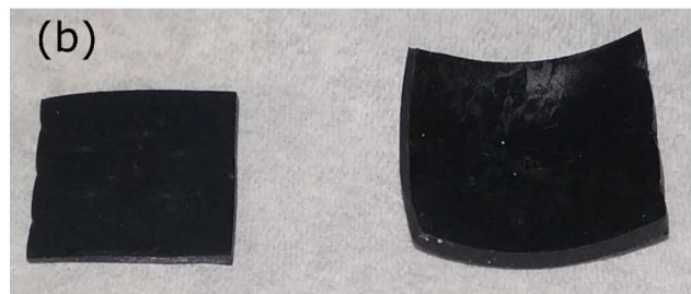
Figure 1. (a) Average weight change for materials in propylene carbonate (PC) after 24 h, 1 week, and 4 weeks in solution. Inset shows exceptional weight change for Viton. (b) Viton before and after soaking.
