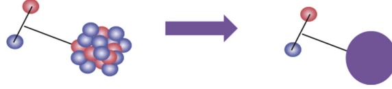
Figure 5. Few-body techniques rely on the reduction of the scattering problem, inherently a many-body problem, to a problem involving only a few relevant degrees of freedom.
