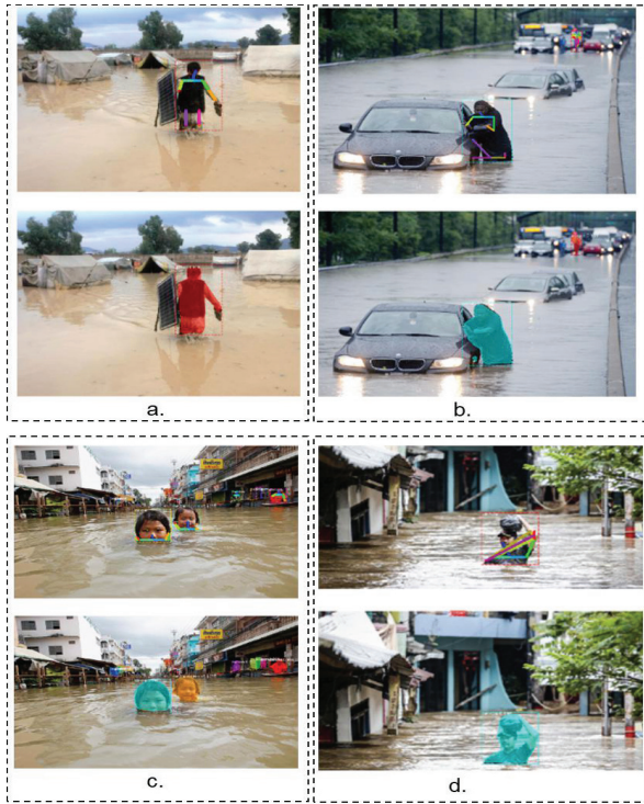
Figure 5. Human keypoint detection for four selected images: only image a generate the correct keypoints
