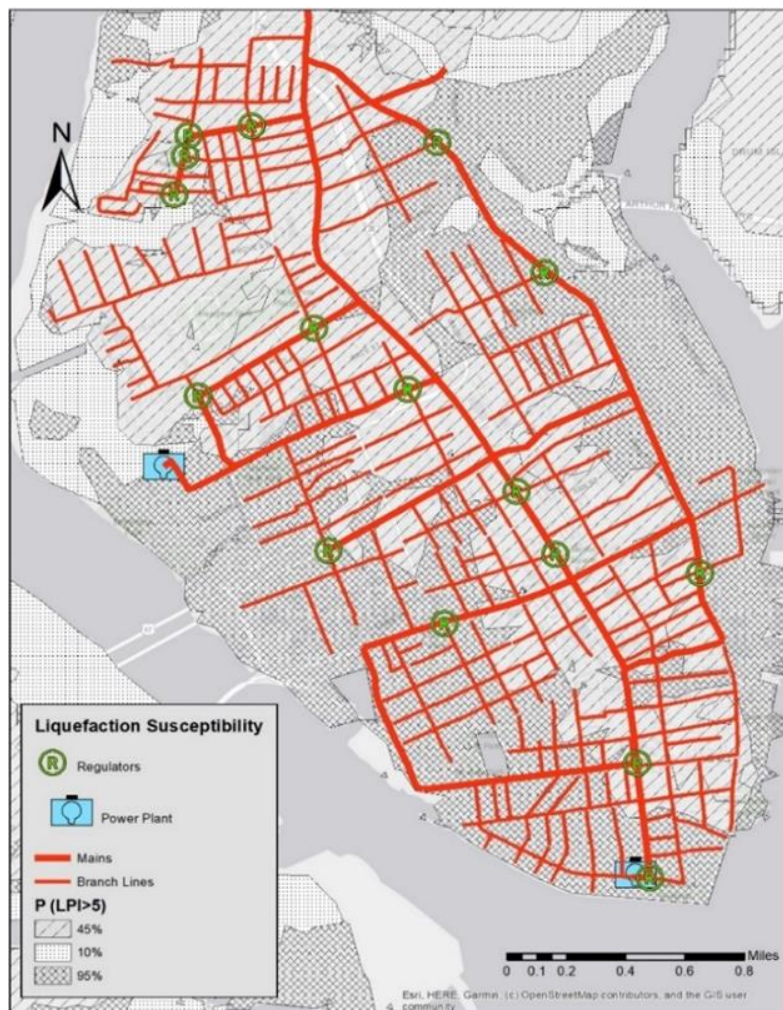
Figure 2. Liquefaction potential map and the hypothetical gas distribution network. Liquefaction map is adopted from (Hayati and Andrus 2008)
