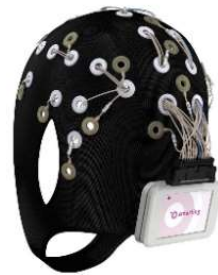
FIGURE 1 – MOBILE EEG CAP WITH 24 CHANNELS AND CORRESPONDING ELECTRODE LAYOUT. ELECTRODES OF INTEREST ARE CIRCLED. SEE SECTION 3.2 FOR MORE INFORMATION ABOUT THESE ELECTRODES. (TAKEN FROM [30]).
