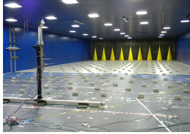
(a) Setup of the experiment to characterize the ABL at PoliMi
