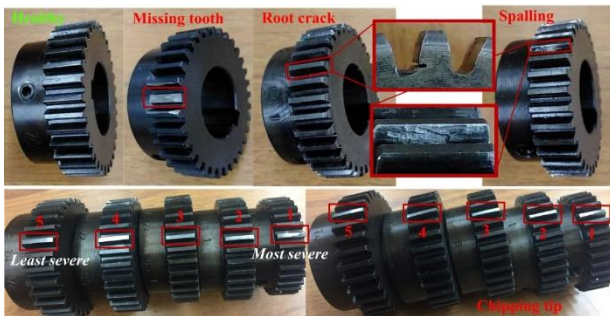
FIGURE 3: 9 PINIONS WITH DIFFERENT HEALTH CONDITIONS (5 SEVERITIES FOR CHIPPING TIP).
