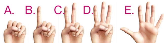
Fig. 5. Leap Motion hand gestures to direct drones. (A) send drone; (B) land drone; (C) change drone altitude (low altitude); (D) change drone altitude (high altitude); (E) search area.
