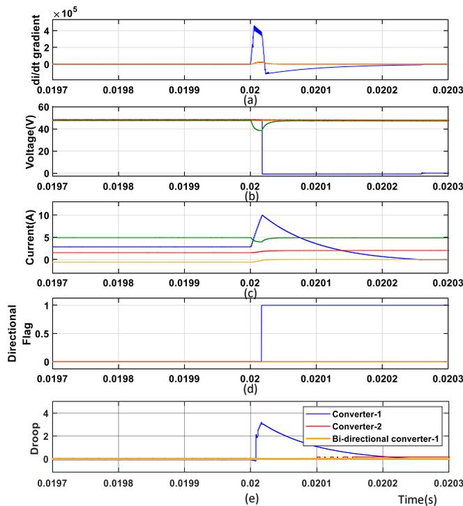
Fig. 11. Bus#1 converter's results for L-L fault  $F_1$  with  $R_f=1 \Omega$  at 0.02 s (a)  $di/dt$  gradients (b) Output voltages (c) Output currents (d) Directional flags, and (e) Calculated adaptive droop values. [Blue  $\rightarrow$  Converter-1, Red  $\rightarrow$  Converter-2, Yellow  $\rightarrow$  Bi-directional Converter, and Green  $\rightarrow$  Load Current]
