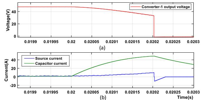
Fig. 13. Converter-1 results for fault  $F_1$  at 0.02 s without proposed algorithm (a) Output voltage (b) Source and capacitor currents.
