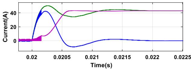
Fig. 4. Fault current contribution of converter-1 during  $F_1$ . [Blue → Capacitor Current, Violet → Source Current, and Green → Output Current]
