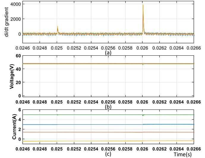
Fig. 20. Results for high impedance feeder fault  $F_3$  at 0.025 s (a)  $\frac{di}{dt}$  gradients (b) Output voltages, and (c) Output currents. [Blue → Converter-1, Red→ Converter-2, Yellow→ Bi-directional Converter, and Green→ Load Current]
