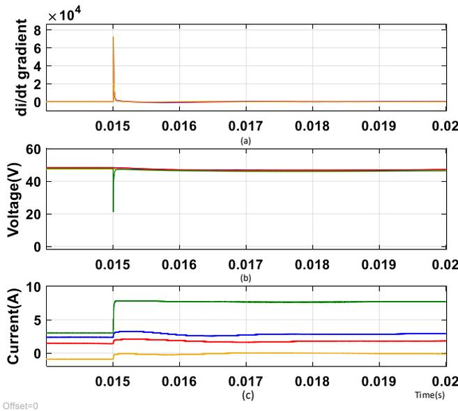
Fig. 23. Simulation results for a step change in bus#1 load at 0.025 s (a)  $\frac{di}{dt}$  gradients (b) Output voltages (c) Output currents, and (d) Current direction/difference flags. [Blue  $\rightarrow$  Converter-1, Red  $\rightarrow$  Converter-2, Yellow  $\rightarrow$  Bi-directional Converter, and Green  $\rightarrow$  Load Current]
