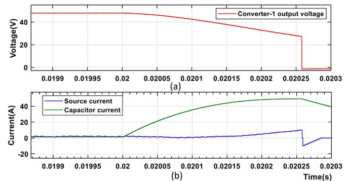
Fig. 14. Converter-1 results for fault  $F_1$  at 0.02 s at 0.02 s with proposed algorithm (a) Output voltage, and (b) Source and capacitor currents.
