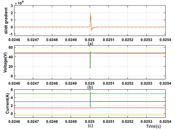
Fig. 17. Results for converter's at bus#1 for a low impedance line-line feeder fault  $F_2$  at 0.025 s (a)  $\frac{di}{dt}$  gradients (b) Output voltages, and (c) Output currents. [Blue  $\rightarrow$  Converter-1, Red  $\rightarrow$  Converter-2, Yellow  $\rightarrow$  Bi-directional Converter, and Green  $\rightarrow$  Load Current]
