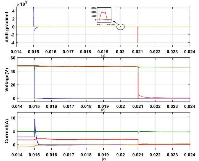
Fig. 21. Simulation results for a combined line-line and line-ground faults at bus#1 Converter's (a)  $\frac{di}{dt}$  gradients (b) Output voltages, and (c) Output currents. [Blue → Converter-1, Red→ Converter-2, Yellow→ Bi-directional Converter, and Green→ Load Current]
