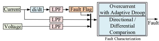
Fig. 7. Proposed DC microgrid fault characterization.
