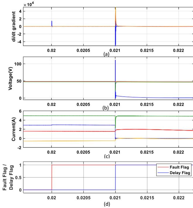
Fig. 18. Results for converter's at bus#1 for a high impedance cable fault  $F_3$  at 0.02 s (a)  $\frac{di}{dt}$  gradients (b) Output voltages (c) Output currents, and (d) Current direction/delay flag. [Blue → Converter-1, Red→ Converter-2, Yellow→ Bi-directional Converter, and Green→ Load Current]
