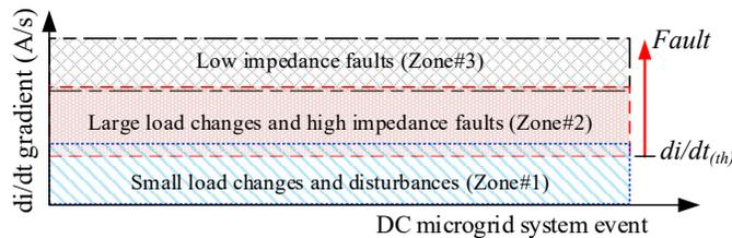
Fig. 6. Classification of system events based on  $\frac{di}{dt}$  gradient.
