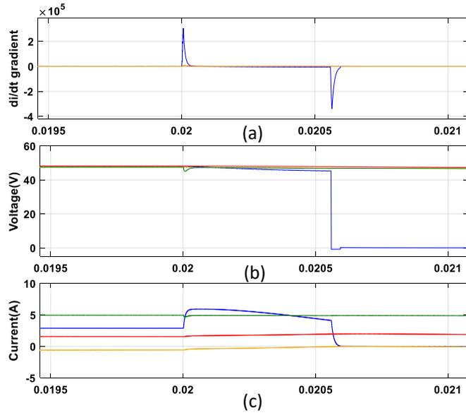
Fig. 15. Bus#1 converter's results for L-L fault ( $F_1$ ) with  $R_f=10\Omega$  at 0.02 s (a)  $\frac{di}{dt}$  gradients (b) Output voltages, and (c) Output currents. [Blue  $\rightarrow$  Converter-1, Red  $\rightarrow$  Converter-2, Yellow  $\rightarrow$  Bi-directional Converter, and Green  $\rightarrow$  Load Current]
