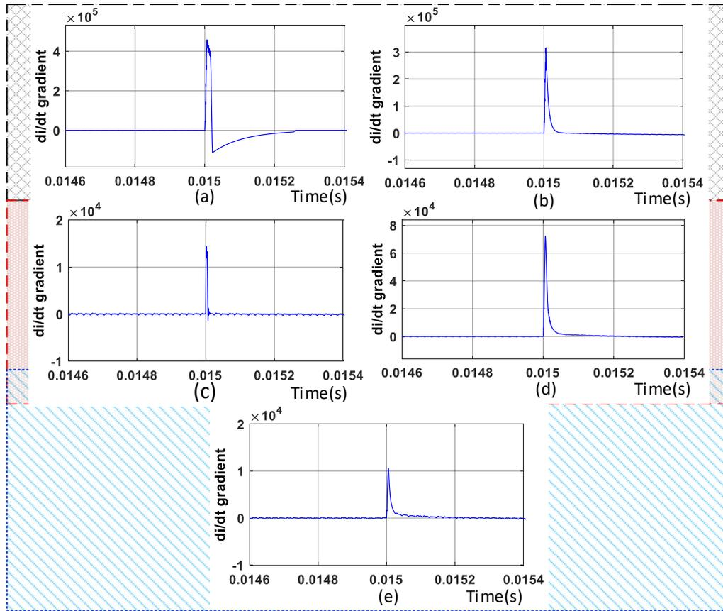
Fig. 5.  $\frac{di}{dt}$  gradient measured for Converter-1 faults and bus#1 load change (a)  $1\Omega$  line-line fault ( $F_1$ ) (b)  $10\Omega$  line-line fault ( $F_1$ ) (c)  $500\Omega$  line-ground fault ( $F_3$ ) (d) Load change from 3 A to 8 A, and (e) Load change from 3 A to 4 A.
