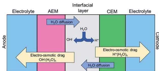
Fig. 8 Diffusion of water to the interface and electro-osmotic drag of water away from the interface.
