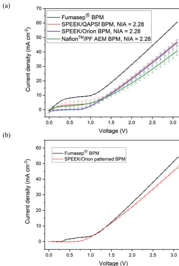
Fig. 6 (a) Polarization curves for micropatterned BPMs with different membrane chemistries. (b) Polarization behavior of Fumasep® and SPEEK/Orion AEM BPMs with the crossover current subtracted.
