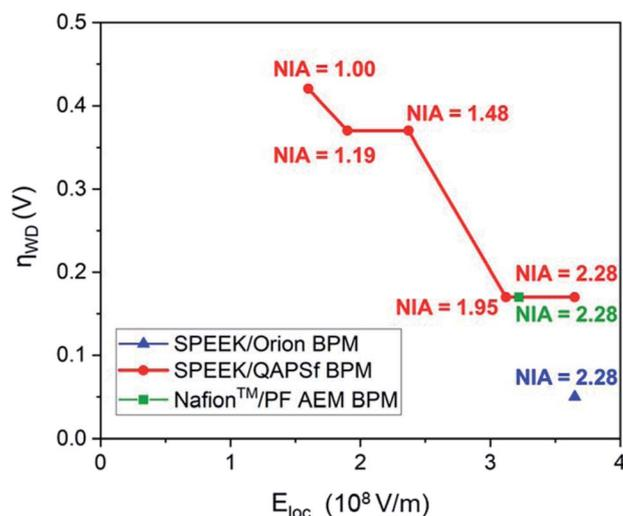
Fig. 7 Onset overpotential for water dissociation as a function of local electric field for various BPMs of varying NIA values and IEC values.
