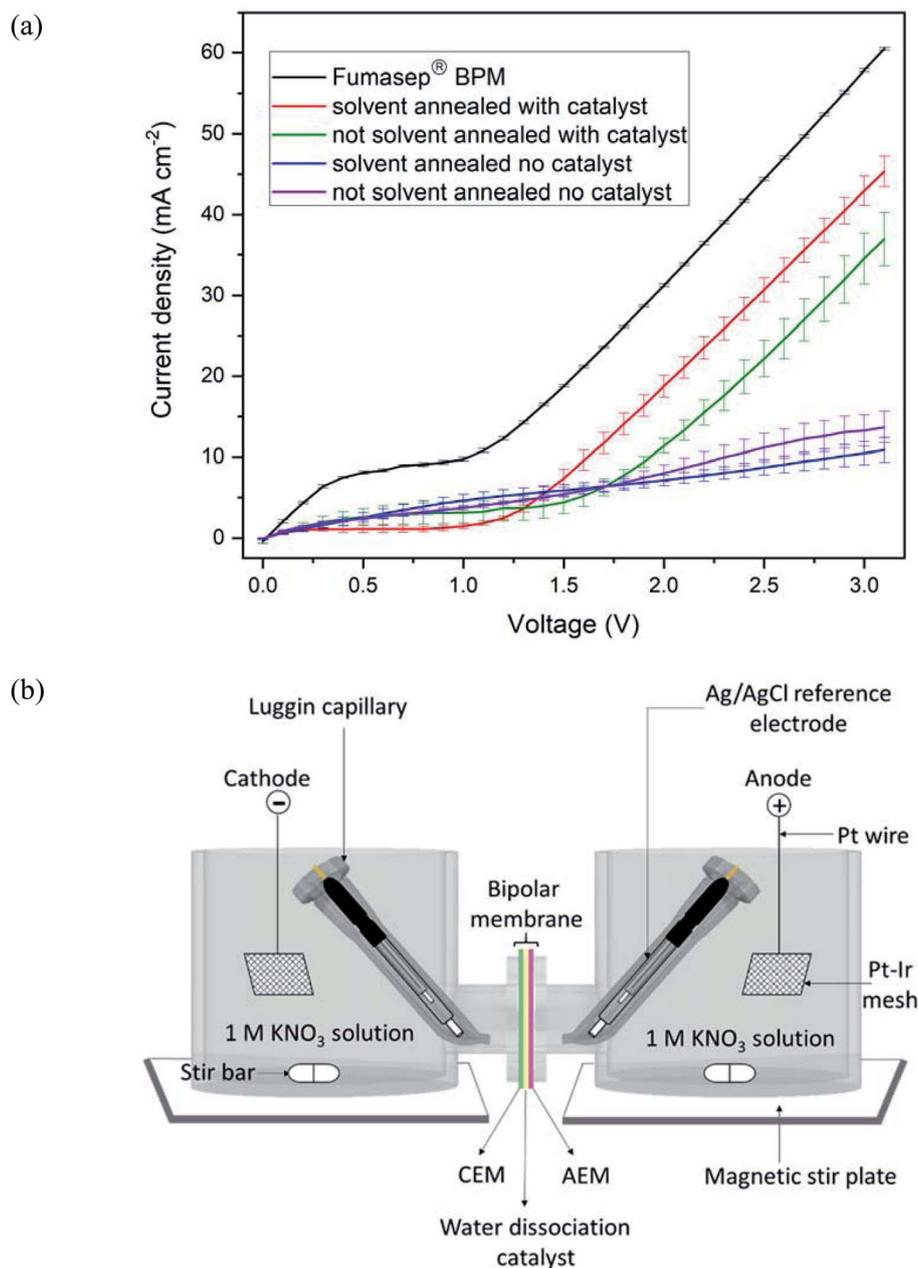
Fig. 3 (a) Polarization curves for non-patterned (*i.e.*, planar interfaces) SPEEK/QAPSF BPMs with and without Al(OH)<sub>3</sub> nanoparticle water dissociation catalysts and with and without solvent vapor annealing processing. Error bars correspond to the standard error for  $n = 3$  independent samples; (b) schematic of the 4-point cell used to evaluate BPM polarization behavior.
