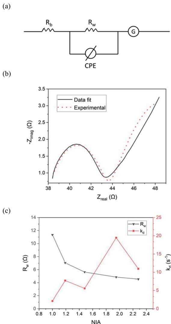
Fig. 5 (a) Electrochemical equivalent circuit (ECE) used to model water dissociation in a BPM. (b) Nyquist plot of representative EIS data of water splitting in SPEEK/QAPSf patterned BPM with ECE model fit (NIA = 1.95). (c) Plot of  $R_w$  and  $k_d^{\text{app}}$  (apparent, forward water dissociation reaction rate constant) versus NIA value.
