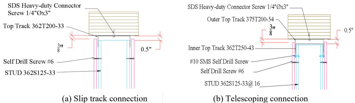
Fig. 3: (a) Slip track and (b) telescoping connection detailing
