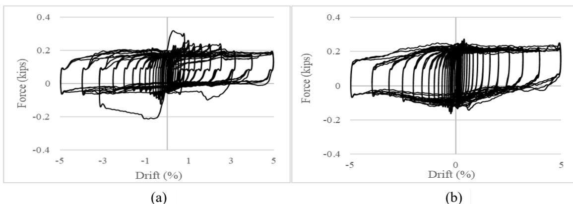
Fig. 13: Phase 1 force vs. displacement hysteresis of drywall partition walls: (a) slip track detailing; (b) telescoping detailing
