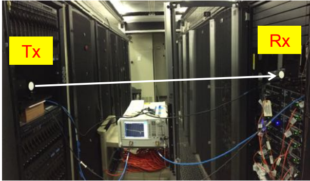
FIGURE 3. Measurement setup for the LoS link at d = 175 cm.
