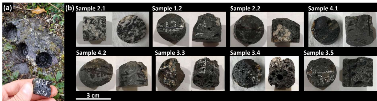
Fig. 2. a) drilled oriented sample with apparent signs of extensive vitrification throughout the entire sample (sample 3.4), and b) all eight oriented samples cut for directional measurements.
