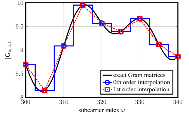
Fig. 1. Illustration of 0th and 1st order interpolation for the entry [\mathbf{G}_\omega]_{1,1} across subcarriers. We explicitly compute the Gram matrix for every fifth subcarrier index \omega and interpolate the remaining matrices. We assume a 128 BS antenna, 8 user massive MU-MIMO system with W = 2048 subcarriers, a delay spread of L = 144 , and perfect CSI without BS-antenna correlation.
