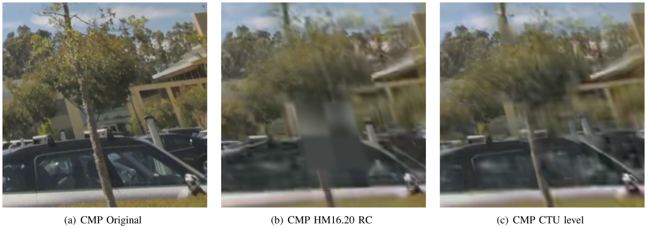
Fig. 8. View port subjective improvement of the CMP format. Test sequence: SkateboardInLot. Picture order count: 9. Configuration: random access. Target bitrate: 2357 kbps. The region shown is a cropped 500 \times 500 zone staring at (1200,1300) from the dynamic view port 0 with size 1816 \times 1816 . (a) original sequence; (b) HM16.20 RC (frame bit cost: 9304); (c) HM16.20 CTU level (frame bit cost: 8696).
