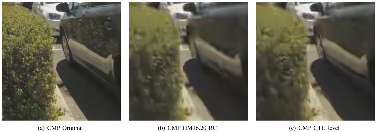
Fig. 9. View port subjective improvement of the CMP format. Test sequence: SkateboardInLot. Picture order count: 165. Configuration: random access. Target bitrate: 2357 kbps. The region shown is a cropped 500 \times 500 zone staring at (1200,1200) from the dynamic view port 0 with size 1816 \times 1816 . (a) original sequence; (b) HM16.20 RC (frame bit cost: 20424); (c) HM16.20 CTU level (frame bit cost: 20304).
