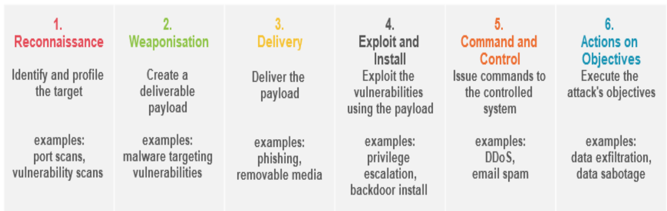
Fig. 2: The cyber attack chain [15]. In the first five steps, the insider acts as a "masquerader" to gain control of the system. The final actions can also be executed by a traitor or an unintentional perpetrator within the organization, skipping the initial steps.
