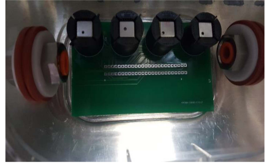
Fig. 2. ZnO/GaN sensor chips with their data collection set-up within gas chamber.
