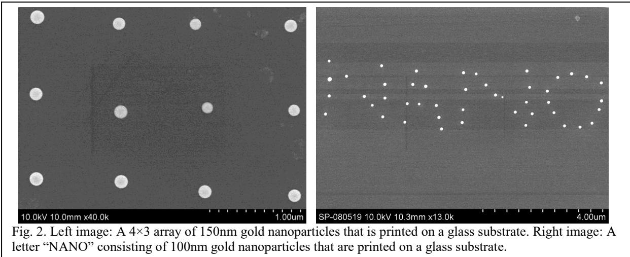
Fig. 2. Left image: A  $4 \times 3$  array of 150nm gold nanoparticles that is printed on a glass substrate. Right image: A letter “NANO” consisting of 100nm gold nanoparticles that are printed on a glass substrate.
