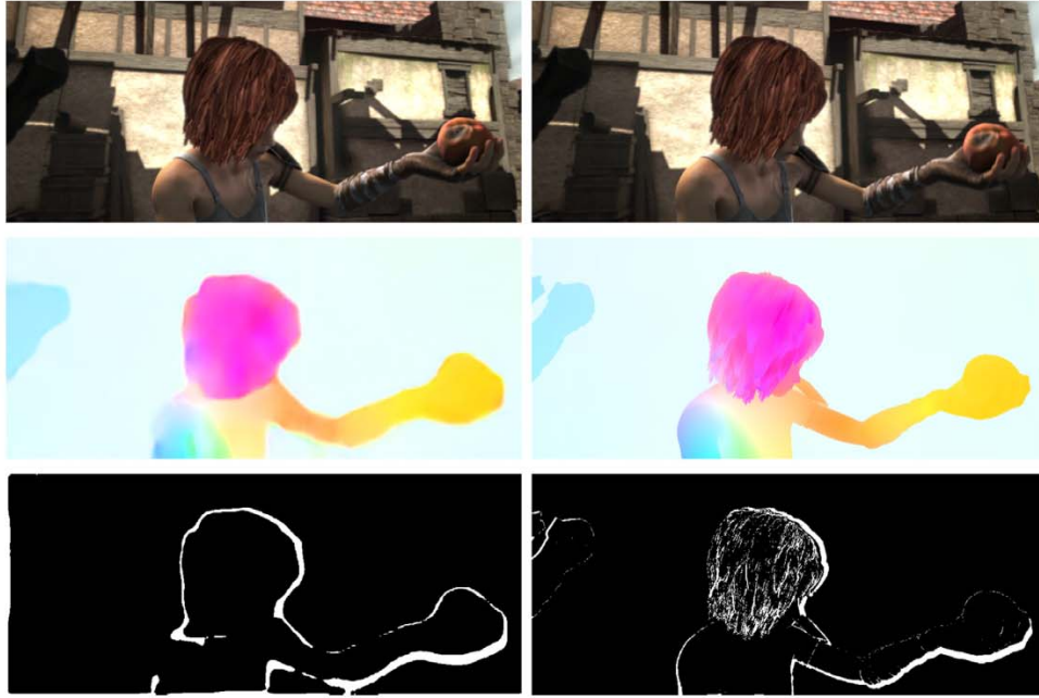
Fig. 6. Qualitative results of our full model method on the MPI-Sintel-final. From the second row to the third row, the left images are the estimated optical flow and occlusion mask respectively. The right images are the corresponding ground truth. The mask is demonstrated by the threshold 0.5.
