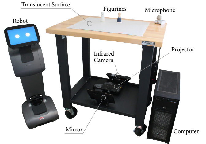
Figure 3: The Figaro system includes the tabletop interface connected to a computer, a tablet control interface, and a robot for deploying designs.
