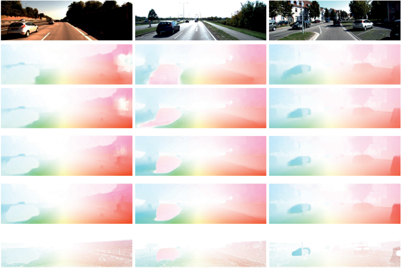
Fig. 4. Qualitative results of the estimated flow fields on KITTI2015 dataset. Original input images are shown at the top row. From the second to the fifth row, the estimation of the initialization, the first round, third round and the fifth round are displayed respectively. Ground truth is shown at the bottom row. The visualization is performed by using the flow visualization protocol in [42].
