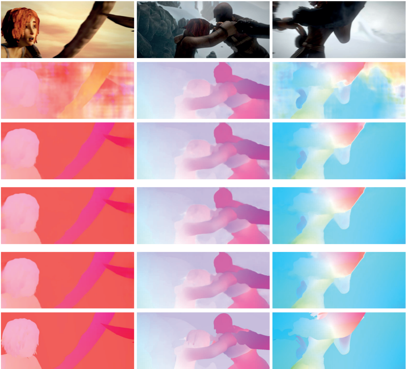
Fig. 5. Qualitative results of the estimated flow fields on MPI-Sintel dataset. Original input images are shown at the top row. From the second to the fifth row, the estimation of the initialization, the first round, third round and the fifth round are displayed respectively. Ground truth is shown at the bottom row. The visualization is performed by using the flow visualization protocol in [42].
