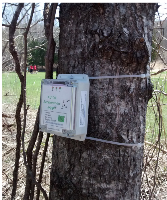
Fig. 1. Accelerometer attached to a balsam poplar ( Populus balsamifera ) tree.
