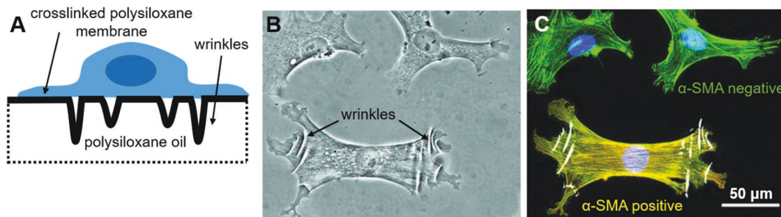
Figure 2. The first seminal method to study cellular forces involved polysiloxane wrinkling. A) Cells were seeded on a polysiloxane fluid that was briefly exposed to a flame to crosslink a thin surface. Cellular forces deformed the membrane and caused it to buckle or wrinkle. B) Wrinkles in the polysiloxane membrane can be visualized under light microscopy. C) When used in conjunction with fluorescent microscopy, the magnitude of cellular forces can be correlated with the expression of biomarkers. For example, a fibroblast that is positive for \alpha -smooth muscle actin (SMA) (yellow) create cellular forces that produce visible wrinkles, unlike those that are negative for \alpha -SMA (green). (B,C) Adapted under the terms of the Creative Commons Attribution 3.0 Unported. [14] Copyright 2001, the Authors. Published by The American Society for Cell Biology.
